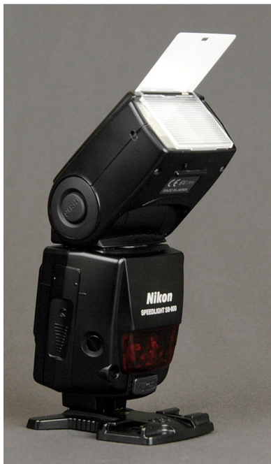
Figure 5.8 When using the Bounce Card, deploy the Wide Angle Adapter for better results. Also, point the flash head upwards at 45 degrees.
