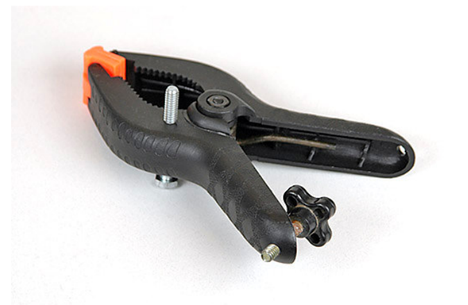
Figure 13.10 I purchase standard plastic clamps from hardware stores and then modify them with 1/4" x 20 bolts so I can mount my flashes to them.
