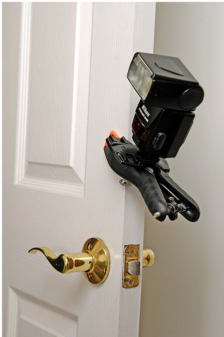
Figure 13.9 Using a simple plastic clamp as shown means you can put a flash just about anywhere! Here, a SB-800 is attached to the clamp with the AS-19 stand that came with the flash.
