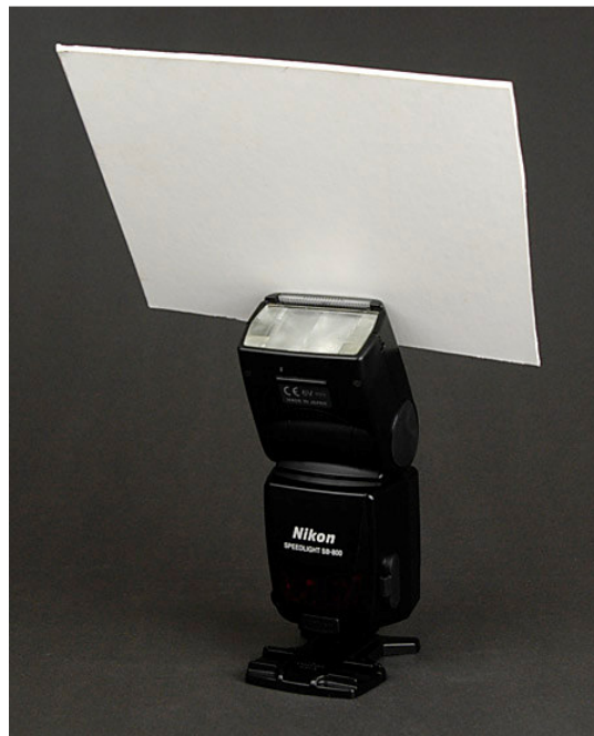
Figure 5.9 This is a "real" bounce card that actually has some useable surface area. It is 5" x 8". The bigger your bounce card the better your flash results! Attach it with Velcro® or Gaffer tape.
